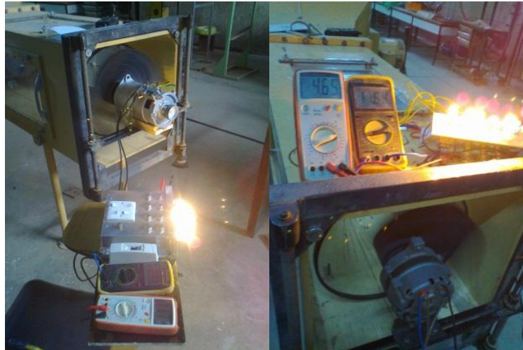
Fig (9): Testing of two generator types, direct DC generator and Alternator
