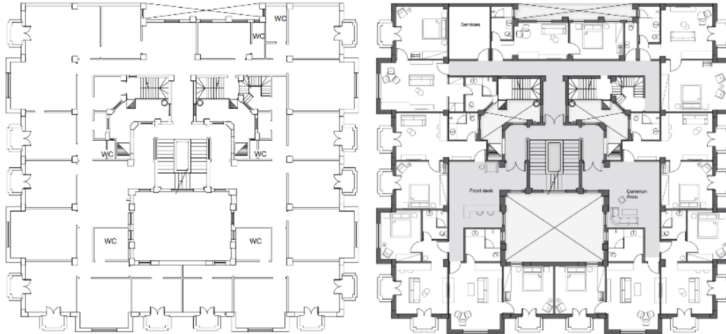
Figure 4. Drawings of floor plans before and after redesign and reuse. Source: Sigma Properties, 2022.
