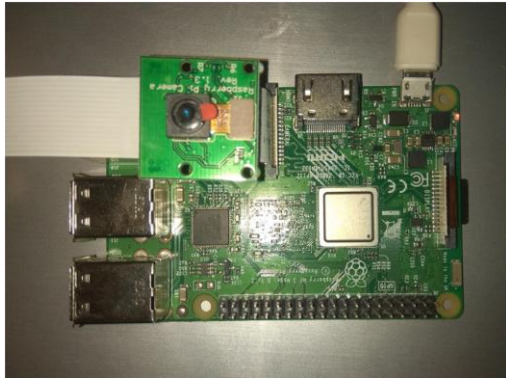
fig.(b): Hardware Design of Sign Language Detection System
